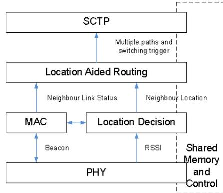
**Fig. 1.** Controlling Flow of the Proposed System
